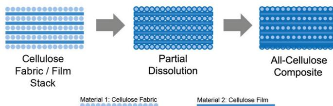
Using this principle, layers of cellulosic material in fabric and film forms can be assembled into a layered stack and dissolved in ionic liquid to create thicker materials that can be formed into three-dimensional shapes.
